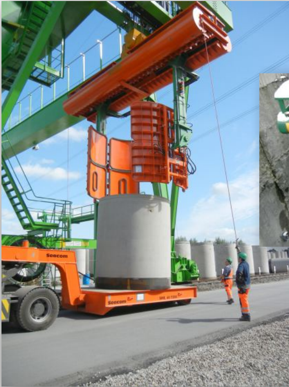
Concrete pipe handling max. 40 t
