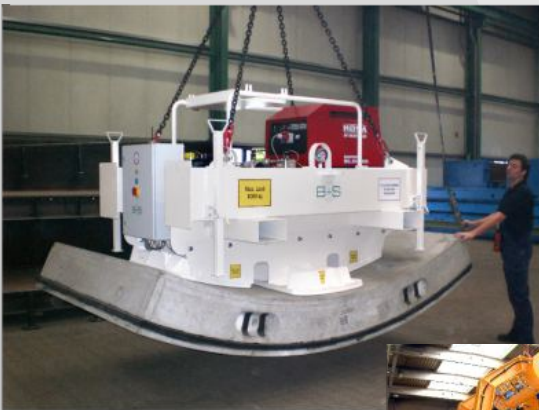
Tunnel segment handling max. 10 t
